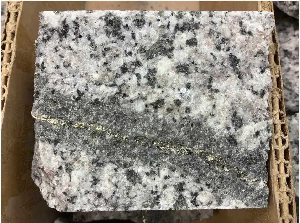
Figure 1: 153m- 1mm wide quartz-pyrite-chalcopyrite vein with biotite-quartz halo
