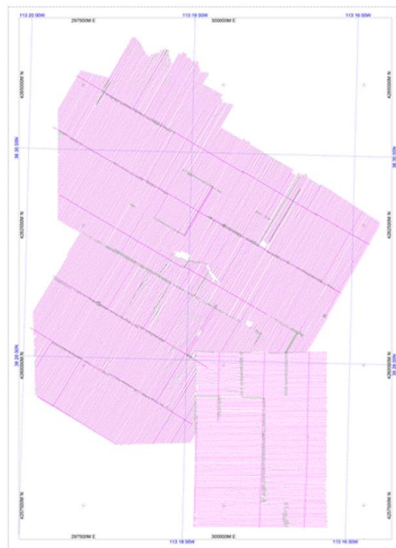
Figure 2. Sawmill Canyon UAV magnetic survey. Magenta points used for final mapping; green points were removed from the survey dataset. Line spacing at 25m. Map provided by MWH.
