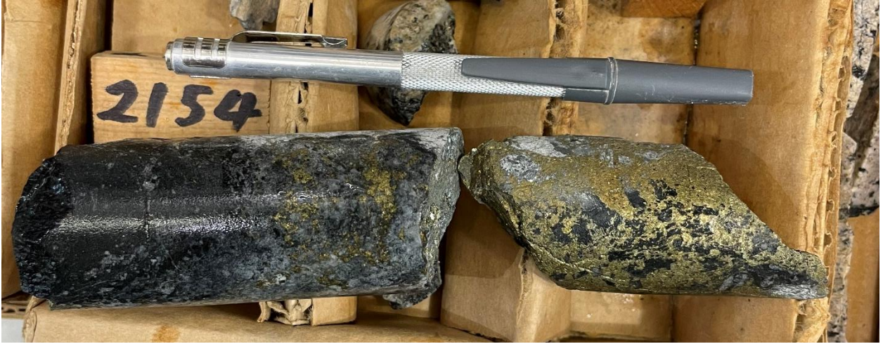
Figure 2: 657m- chalcopyrite-tourmaline-quartz cemented breccia
